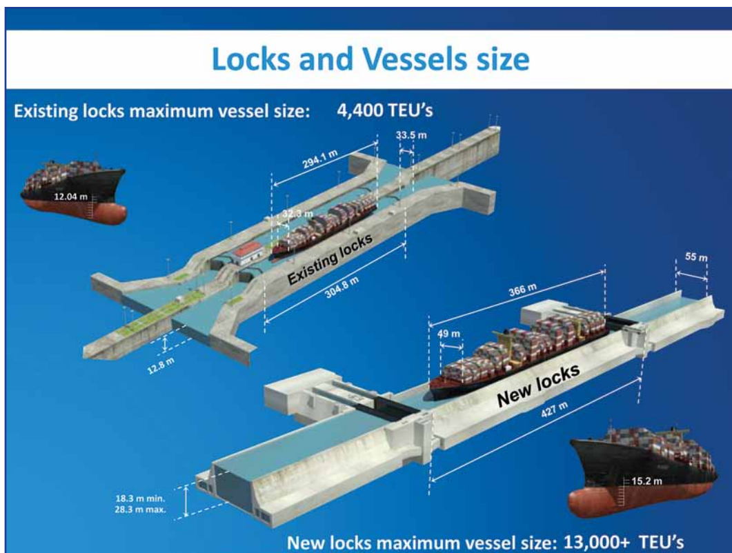
Comparison of existing Panama Canal locks and new Panama Canal locks. Courtesy of the Panama Canal Authority.
