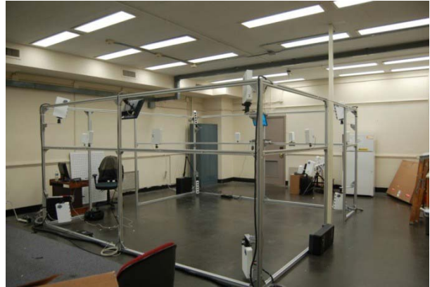
Figure 1: Whole Body Scanner Set-Up
