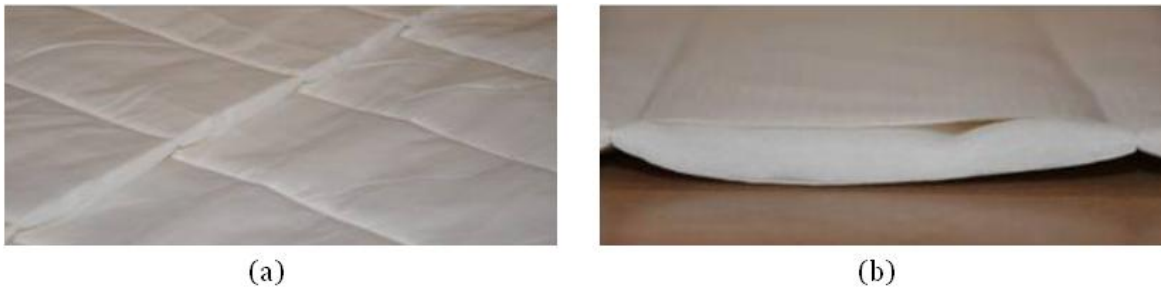
Figure 2-4. Nonwoven Insulation liner, (a) manufacturing quilt lines of current prototype liner system, (b) fibrous batting.
