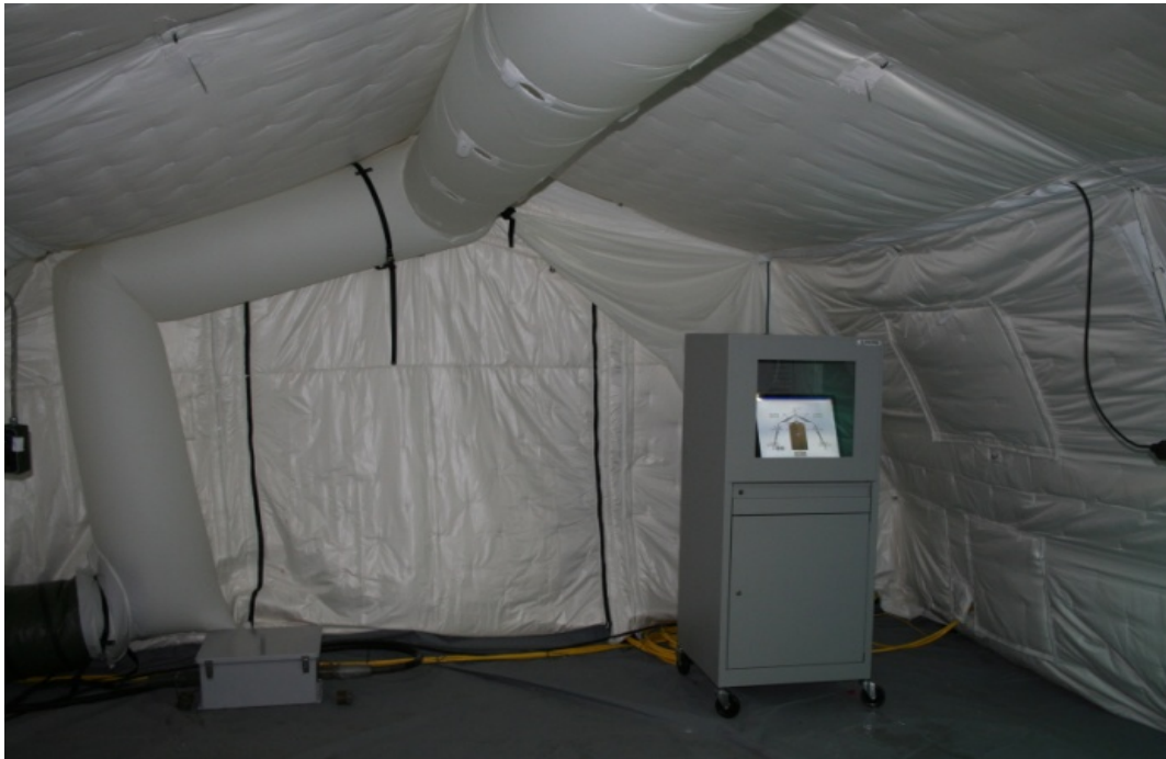
Figure 2-2. Utilis TM60 shelter with nonwoven composite insulation (Thinsulate™) liner (Camel Manufacturing, Pioneer, TN).
