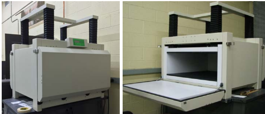
Figure 3-4. Laser Comp 801 HFMA for measuring thermal conductivity and determining R-values of insulation (Left: outside closed HFMA, Right: Inside of HFMA).
