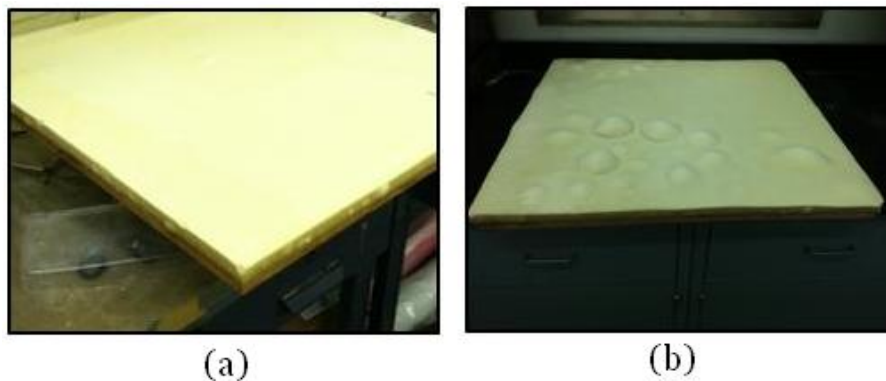
Figure 4-3. Blistering occurs on ccSPF samples: (a) typical blistering shown on edges of ccSPF sample, (b) severe blistering shown on top of ccSPF sample.
