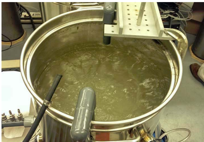
Figure 26. Photograph of 5% acetic acid solution in the leaching system.
