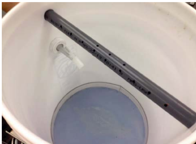
Figure 21. Interior of the leach heap tank. Spray bar was turned to show detail.
