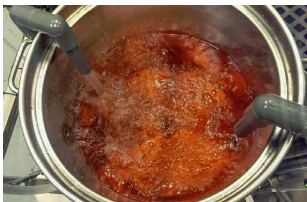
Figure 16. Mixing of food-grade color concentrate in batch mixing tank.
