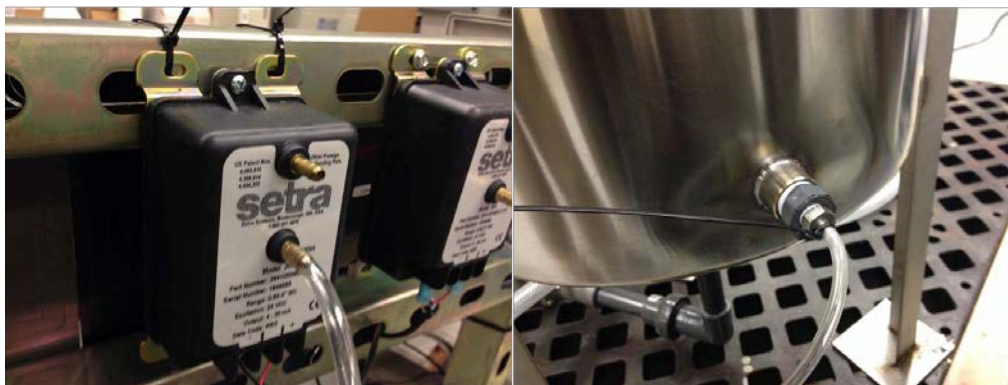
Figure 11. Pressure sensors for measuring tank volumes.
