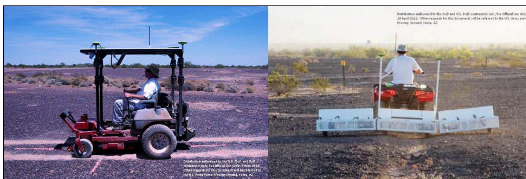
Figure 1. Photographs of the 1-meter-wide surveying system (left) and the 3-meter-wide surveying system (right).
