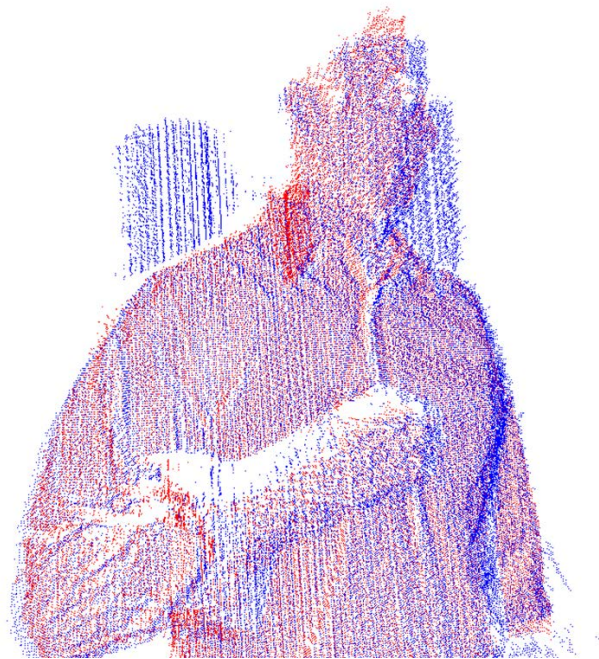
Figure 3.11: Merged camera A (red) and B (blue) points clouds resulting from unwrapped phases of Fig. 3.9.
