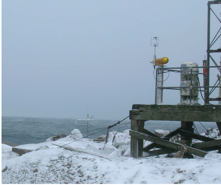
Figure 5. The cloud imaging probe (gold instrument) and its associated sonic anemometer/thermometer (thin instrument with several short arms near it) on the foghorn platform at Mt. Desert Rock in January 2013. The laser array is on the far end of the probe on the thin, gold arm that is barely visible. The sonic anemometer is crucial for evaluating spray concentration from the cloud imaging probe’s measurements because it provides the direction and speed of the drops through the laser array.
