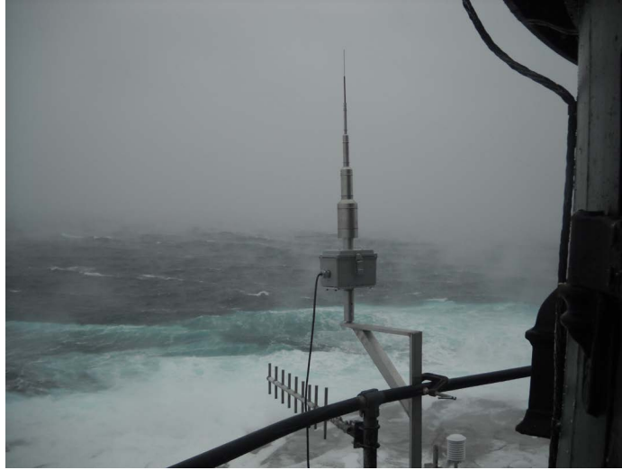
Figure 2. Rotating multicylinder observation on the lower catwalk on the lighthouse, 22 Jan 2014. The wind and the mass of ice on each cylinder are analyzed to determine the best fit parameters of an assumed drop concentration distribution.
