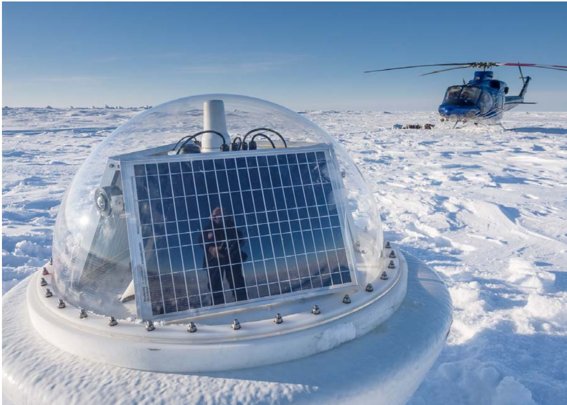
Figure 1: One of the solar-powered wavebuoys deployed on ice from the Sachs Harbour ice camps
