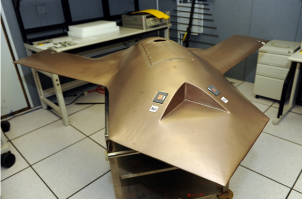
Fig. 1: UCAV with square patch antennas.
