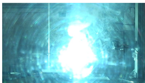
Figure 5. \text{ZrB}_2/\text{KNO}_3 green flame (see Table 4b).
