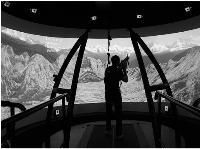
Fig. 1. The Physical and Cognitive Operational Research Environment (PhyCORE), which provides an interactive, immersive environment for use in diagnostics, rehabilitation, and research.
