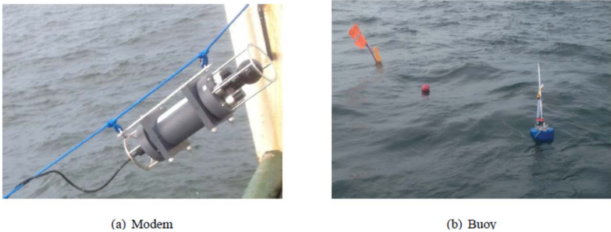
Figure 4. The OFDM-modulated dynamic coded cooperation experiment, May 2013. (a) The OFDM modem before entering the water during deployment; (b) The buoy after being deployed
