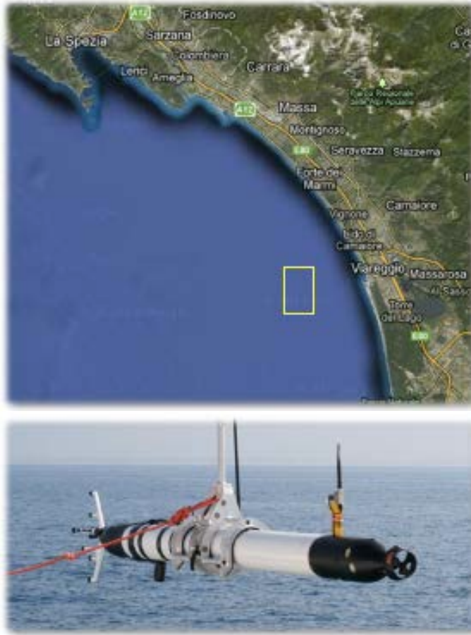
Figure 6. Upper Panel: Location of the Glider Acoustic Sensing of Sediments (GLASS) experiment off the coast of Italy. Lower Panel: The Folaga glider equipped with the GLASS hydrophone array on the bow.
