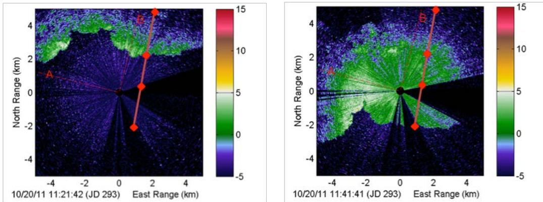
**Figure 9: Surface aerosol backscatter from horizontal scans with edge tracking results (in red). These two scans, separated by 20 minutes in time, show the propagation of the leading edge of the outflow.**
