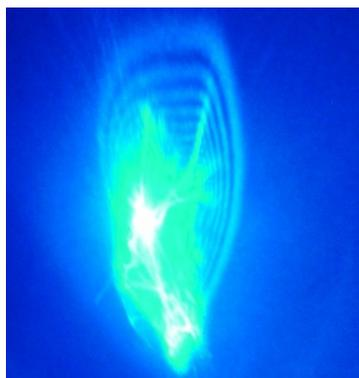
Fig.11. Nonlinear reflection of the blue laser light from the border of the oil film-water interface. The bright spot in the center is the reflection from the water, interference fringes are from the oil film, and the green light is due to fluorescence.
