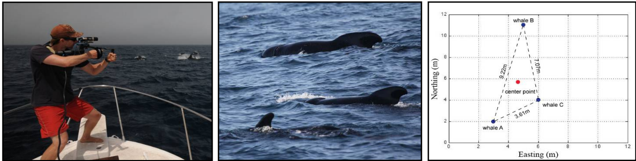
Figure 4: The current stereo geocoding system for 3D localization of whales and quantification of social group cohesion. Left: Example of stereo camera system used in August 2012 field cruise, sampling at 4 Hz. Center: Image of 3 pilot whales similar to what is captured by a single of the two cameras. Images from both cameras are analysed to find a distance to different whales using the known aperture and calibration values, and then combined with the GPS position and pointing vector of the camera to calculate georeferenced positions. Right: Conceptual illustration of geocoded position estimates of the three animals shown on image in the bottom left. An initial RMS measure of social group cohesion could be derived as the root-mean-squared distance from each whale (dorsal fin location shown in blue circles) to the mean group position (red circle), for a mean group spread of 4.05 m in this example, and with individual distances between animals noted on figure. Range resolution for the current system is better than \pm 1m at 50 meters distance.
