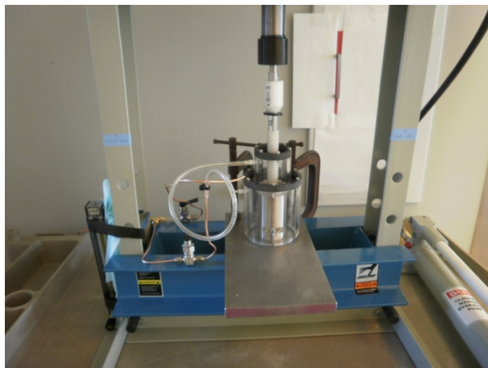
Fig. 4: Device for anaerobic excision and grinding of tissue
