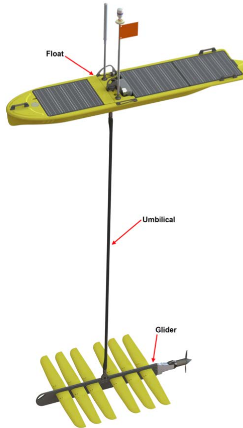
Figure 1. Wave Glider components: Float and sub separated by a 4 m umbilical
