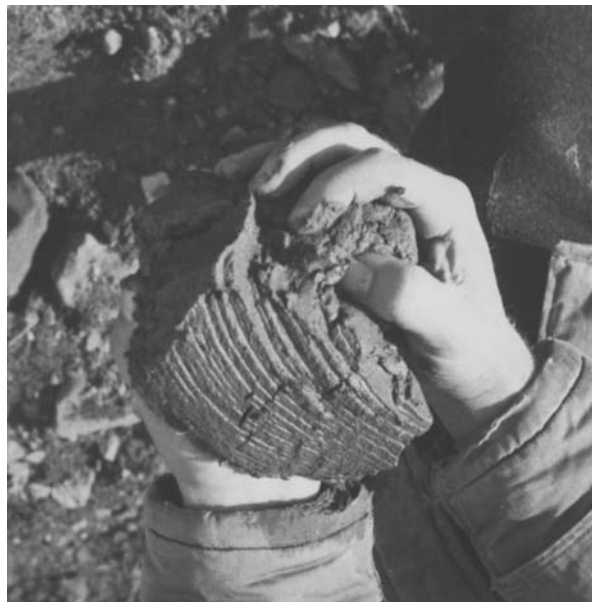
Figure 7: Image of the varved sediment that accumulates on the banks of the Petitcodiac River at Moncton during periods of rapid accumulation. The varves separate along a coarse silt layer.
