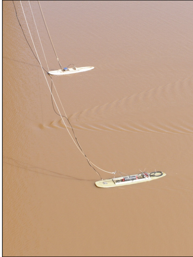
Figure 2: Photo of the instrumented surfboards deployed from the bridge in the Petitcodiac River. Upper board consists of a 1.2 MHz RDI ADCP and a Dual Frequency (50 and 200 kHz) Knudsen echosounder. The lower board has a 2.5 MHz rotary sonar and 1.2 MHz RDI ADCP mounted on it. The wake between the boards is caused by a SUBS package just below the surface.
