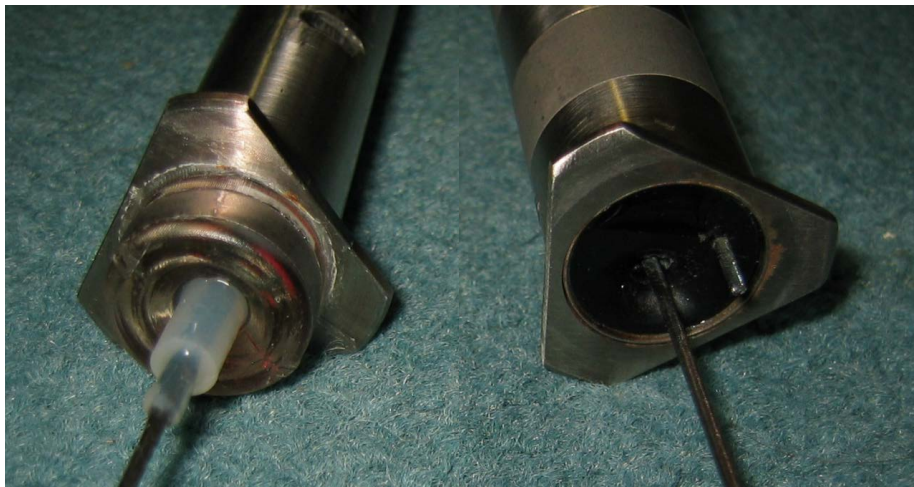
Fig. 2 – Design modifications in the posterior end of implantable satellite tags. The previous design with an exposed epoxy bulb is shown on the left while the new model with a flush posterior end and with the wet/dry sensor (salt-water switch) represented by a Nitinol cable is shown on the right.
