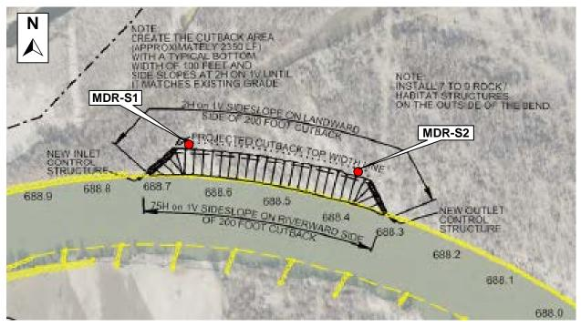
Figure 2. Location of sediment/soil sampling sites at the proposed Middle Decatur Revetment project site.
