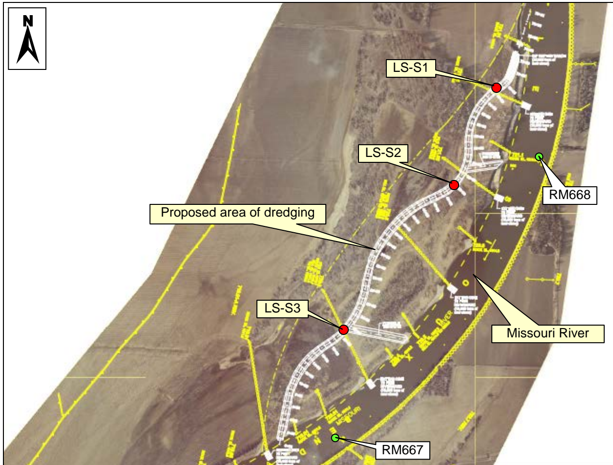
Figure 2. Proposed excavation to create shallow-water habitat at the Little Sioux project area.
