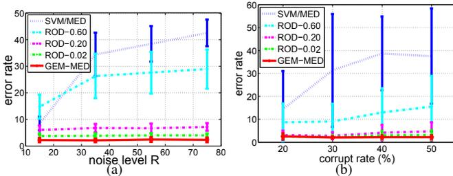
**Fig. 1:** (a) Test error (%) vs. noise level  $R$  (corruption rate = 0.2). (b) Test error (%) vs. corrupt rate ( $R = 55$ ) on simulated data. GEM-MED outperforms both MED/SVM and ROD for various  $\rho$  in classification accuracy, when either noise level or corrupt rate increases .
