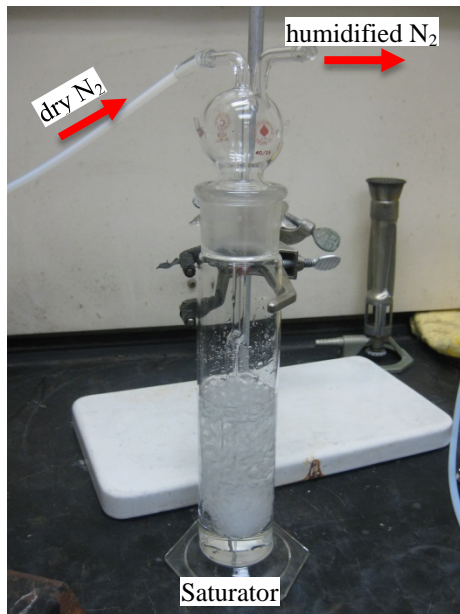
Figure 3 Humidify the N 2 stream by a saturator.
