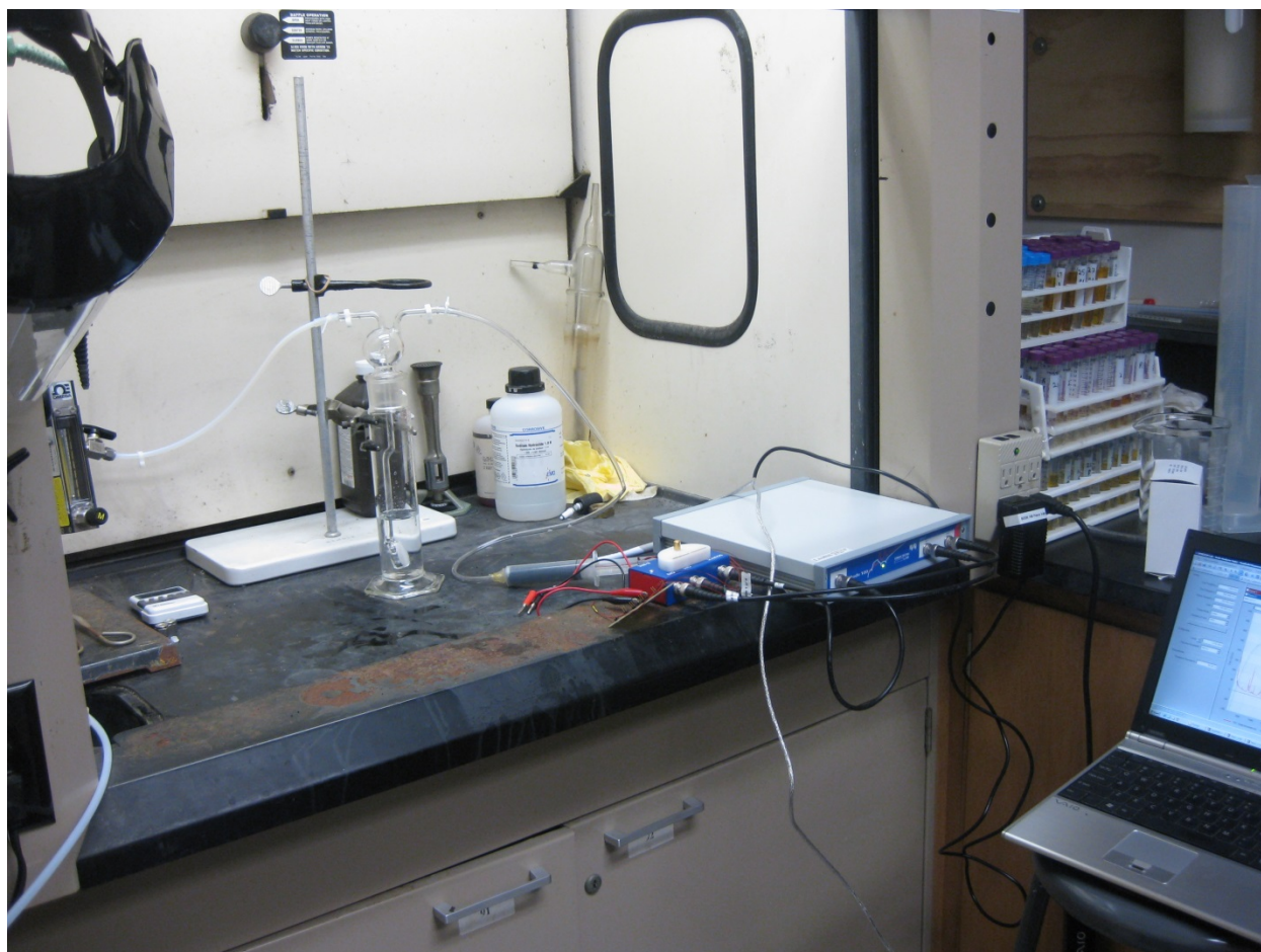
Figure 4 Experimental setup used for the humidity test on carbon bed embedded with PWAS.
