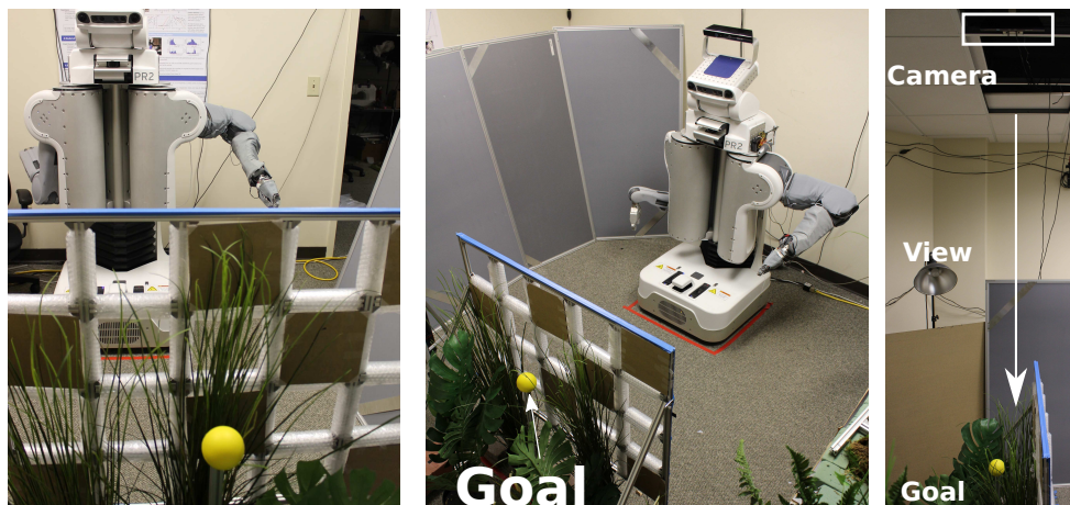
Figure 5: View of a reaching-in-clutter experiment with a PR2 in a foliage-aperture-clutter
