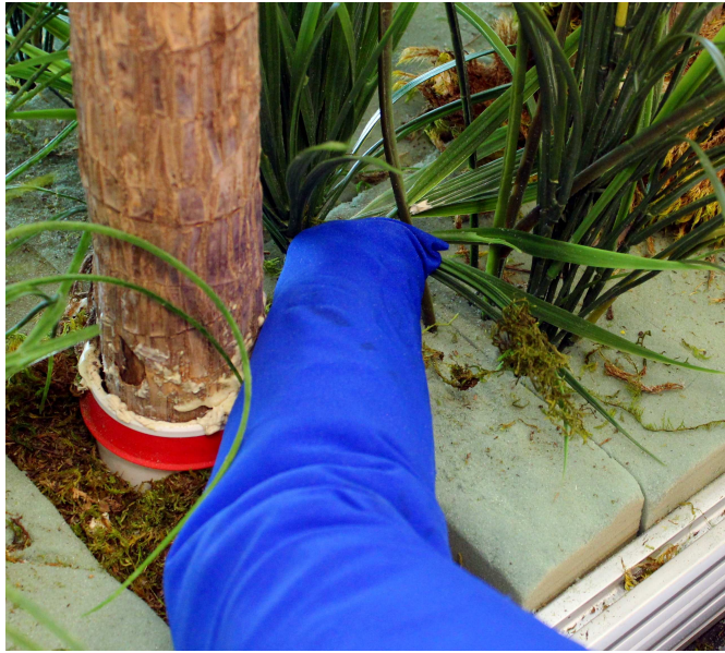
Figure 12: End-effector stuck against foliage and trunk during greedy reach toward goal #5. The leaves of two fake plants have intertwined and created a barrier which the controller will not push through due to force constraints.
