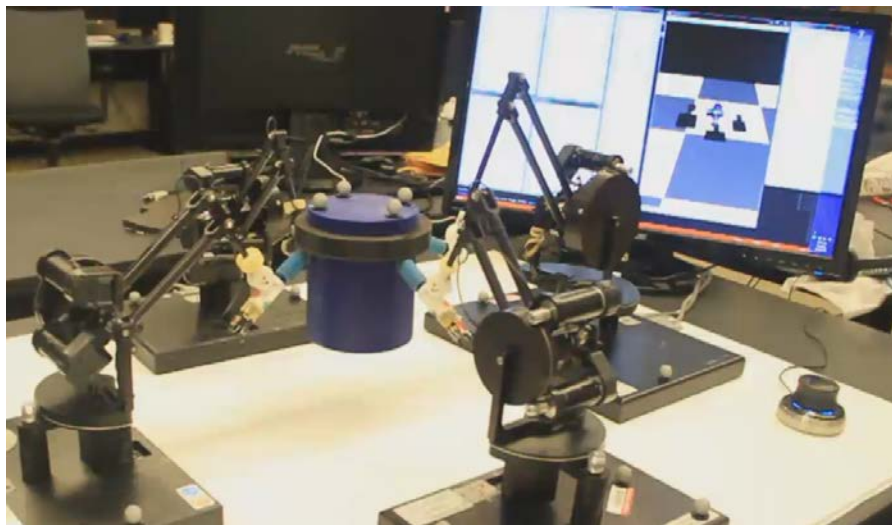
Figure 4. MPC of dexterous object manipulation with a 12-dof "hand" made of 4 Phantom robots. This figure is from Erez et al, submitted to ICRA 2014.
