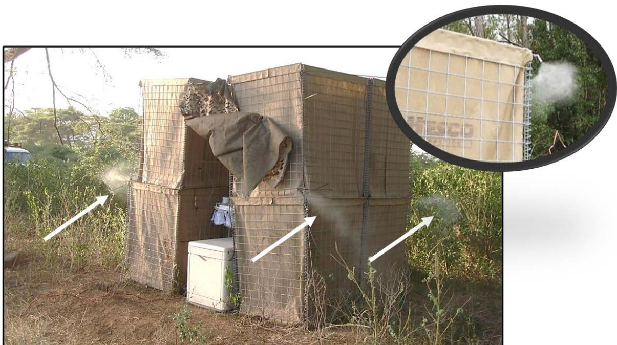
Fig. 6-4. Misting system fitted to experimental HESCO® units targeting sand fly vectors of Leishmania in the Rift Valley, Kenya. Arrows indicate mist plumes; inset shows detail of nozzle and spray. Photo: Seth Britch, USDA.
