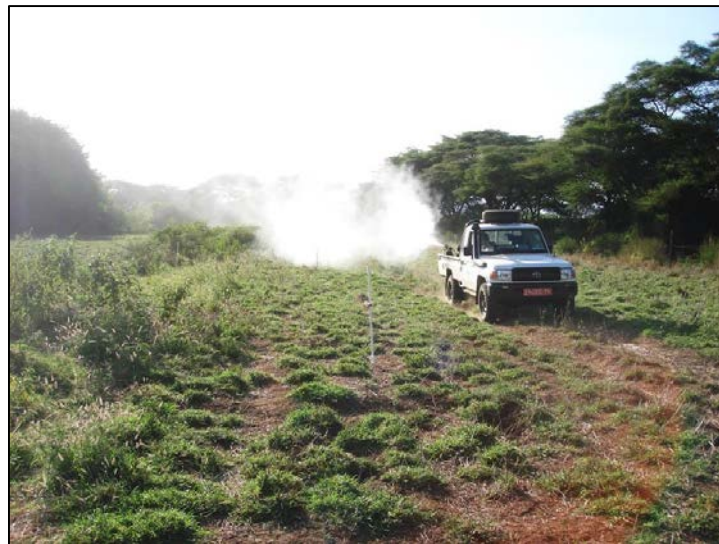
Fig. 6-3. An aerosol application of Duet® (sumithrin, prallethrin, PBO) with a truck-mounted Terminator ULV against sand flies in an experimental plot in the Rift Valley, Kenya. Photo: Seth Britch, USDA.
