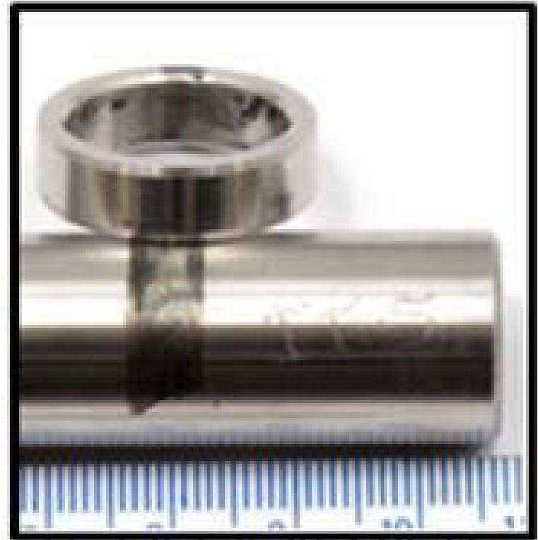
Nano Co-alloy Bushing: 440C Pin 2000 cycles total 400 cycles at 10,000 lbs
