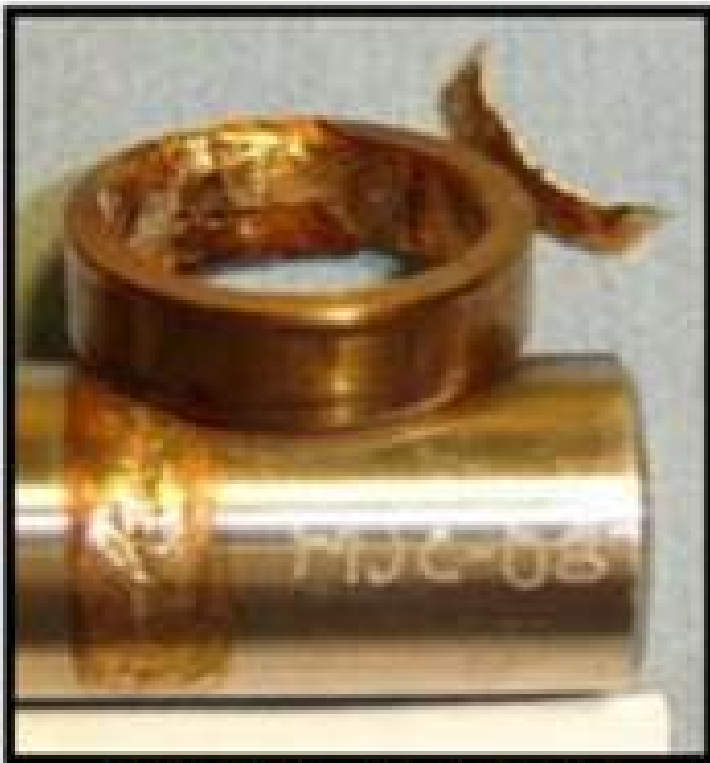
Cu-Be Bushing: MP 35N Pin 1725 cycles total 125 cycles at 10,000 lbs
