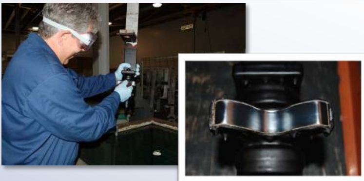
EHC Plating of T-45 Pivot Assy
