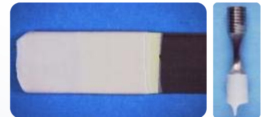
Maskant on Flat Coupons/Threaded items Evaluated at 130°C (266°F)
