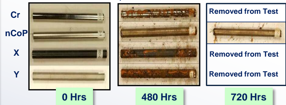
Carburized 1018 Steel Coupons
