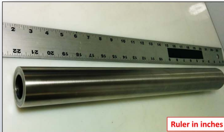
Nanovate™ R3010 Plating on Navy Shaft geometries/materials
