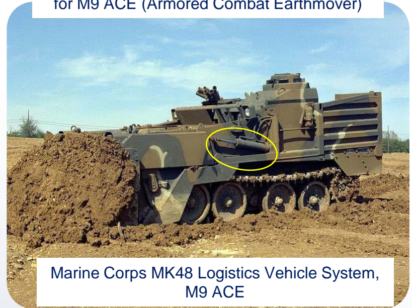
Nanovate™ R3010 plated Hydraulic Cylinder for M9 ACE (Armored Combat Earthmover)
