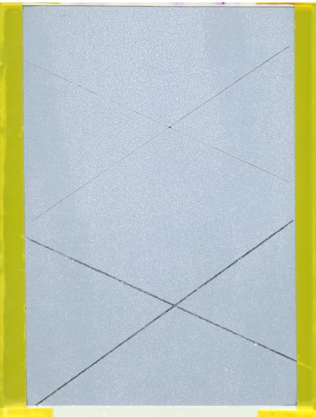
Primed TCP/ZnNi/4130 2,000hrs ASTM B117
