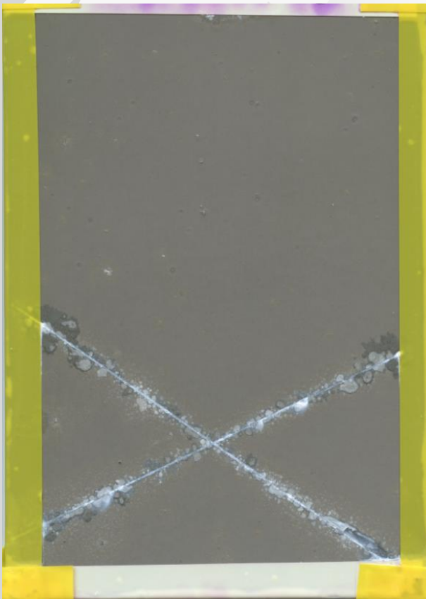
Non-Inhibited primer over TCP/ZnNi/4130 2,000hrs ASTM B117
