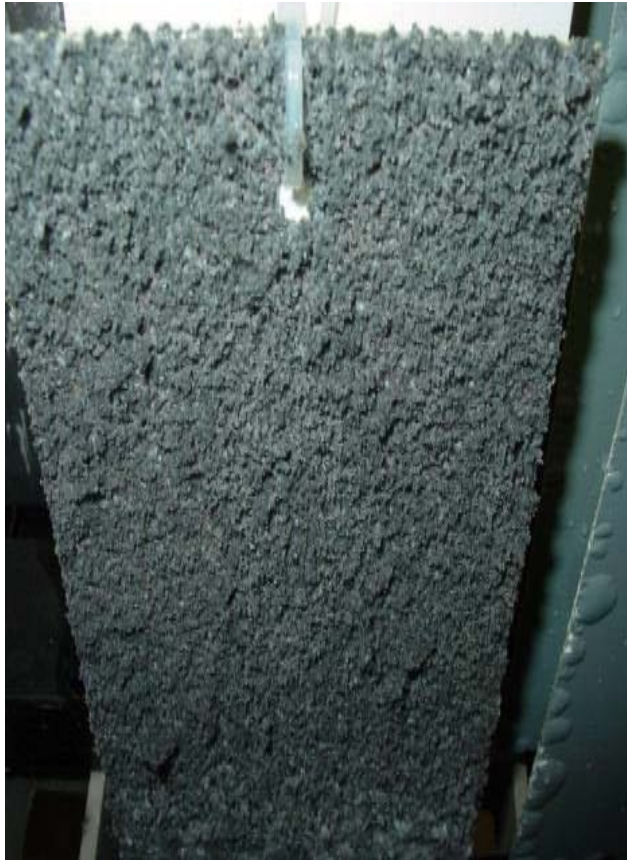
Mg Alloy Panel after 48 hrs.
