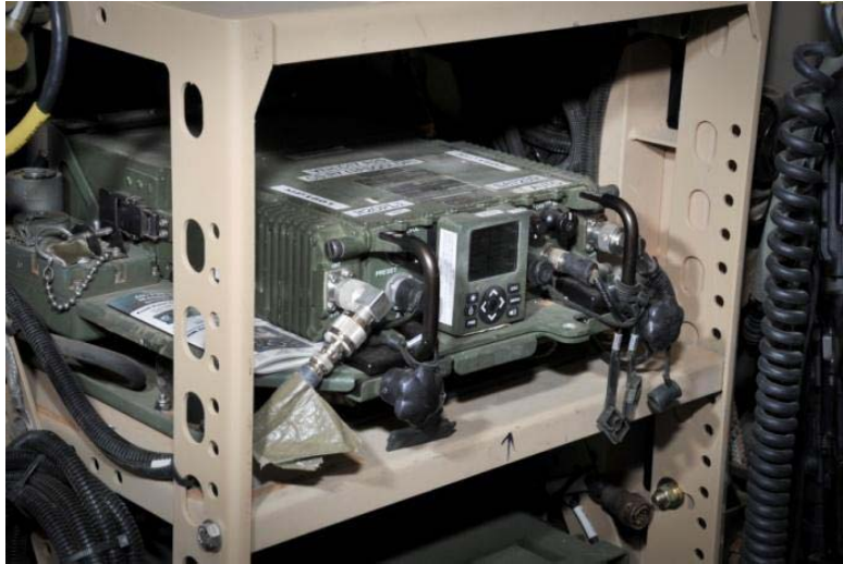
Figure 1-2. HMS Manpack Radio in Vehicle-mounted Configuration
