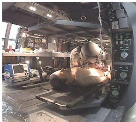
Figure 26. TP A can apply adequate pressure to femoral artery with 26 in. of available vertical space but cannot bandage while maintaining pressure (task 32).
