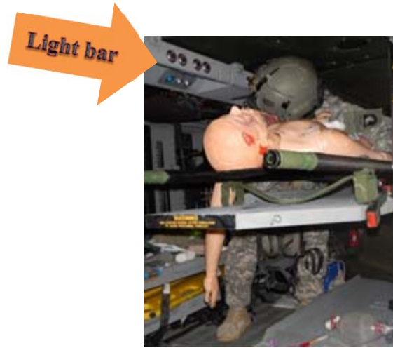
Figure 35. TP 2 unable to complete task 37 with 24 in. vertical clearance in the upper litter position during Phase 3.
