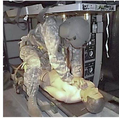
Figure 33. TP C1 able to fully extend arms and lock elbows to successfully complete task 27 with 37 in. of vertical space.
