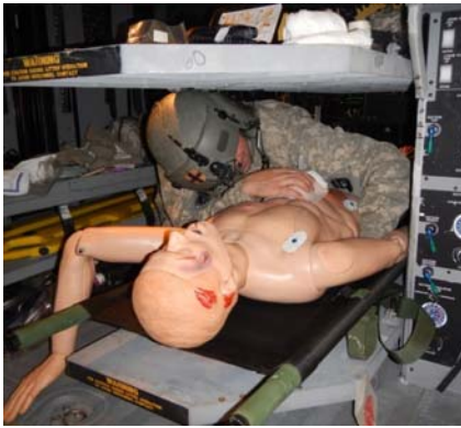
Figure 34. TP 2 able to complete task 37 with 24 in. vertical clearance in the lower litter position during Phase 3.
