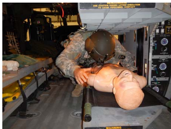
Figure 36. TP 15 required 25 in. of vertical space to complete task 32.
