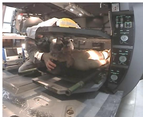
Figure 27. TP A with 18 in. of vertical spacing cannot insert nasopharyngeal airway because of insufficient line of sight (task 4).
