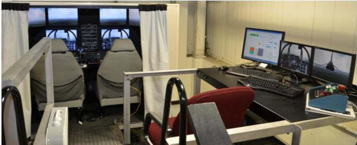
**Figure 1.20.** The WVU 6-DOF Motion-based Flight Simulator
