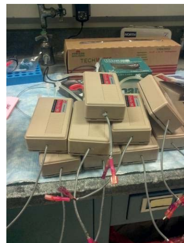
Figure 6. Modified pumps (sealed sample and return lines)
