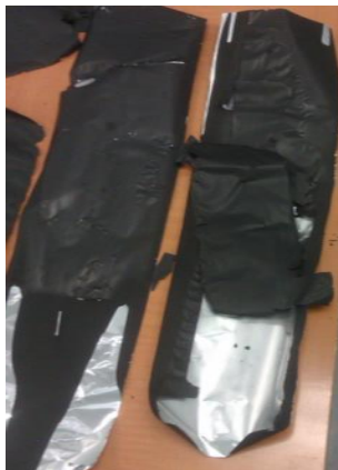
Figure 17 LVP electrodes with high loading, coated using coating machine in the pilot line; material come off after roller pressing.
