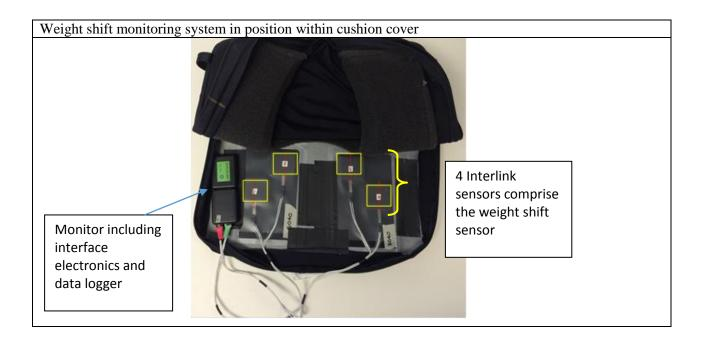
Fabrication of seat sensors, interfacing with data measurement hardware, and sensor characterization.
