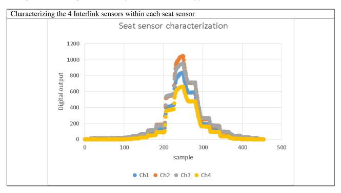
The weight-shift sensor is designed to monitor the loading on a wheelchair cushion. Changes in posture result in changes in load which is measured by the weight shift monitoring system. In order to document the type and frequency of weight shifting behaviors, force data from the sensors must be categorized. This is a difficult challenge and one that is on-going.
