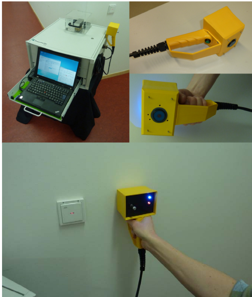
Figure 39. Photo of the High-Frequency Eddy Current Based Testing System
