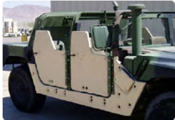
Fig. 4. Polyurea coating to protect military vehicle
