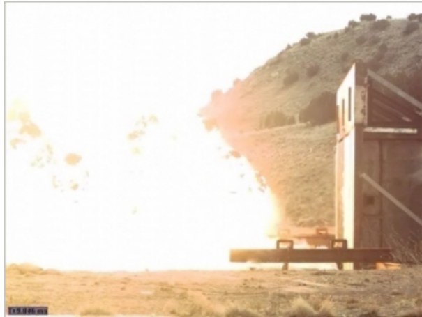
Fig. 2. Blast made in front of the wall
