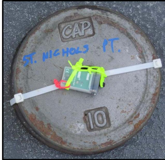
Figure 7. HOBO<sup>®</sup> data logger attached to 10-pound weight so that it did not move with the currents.
