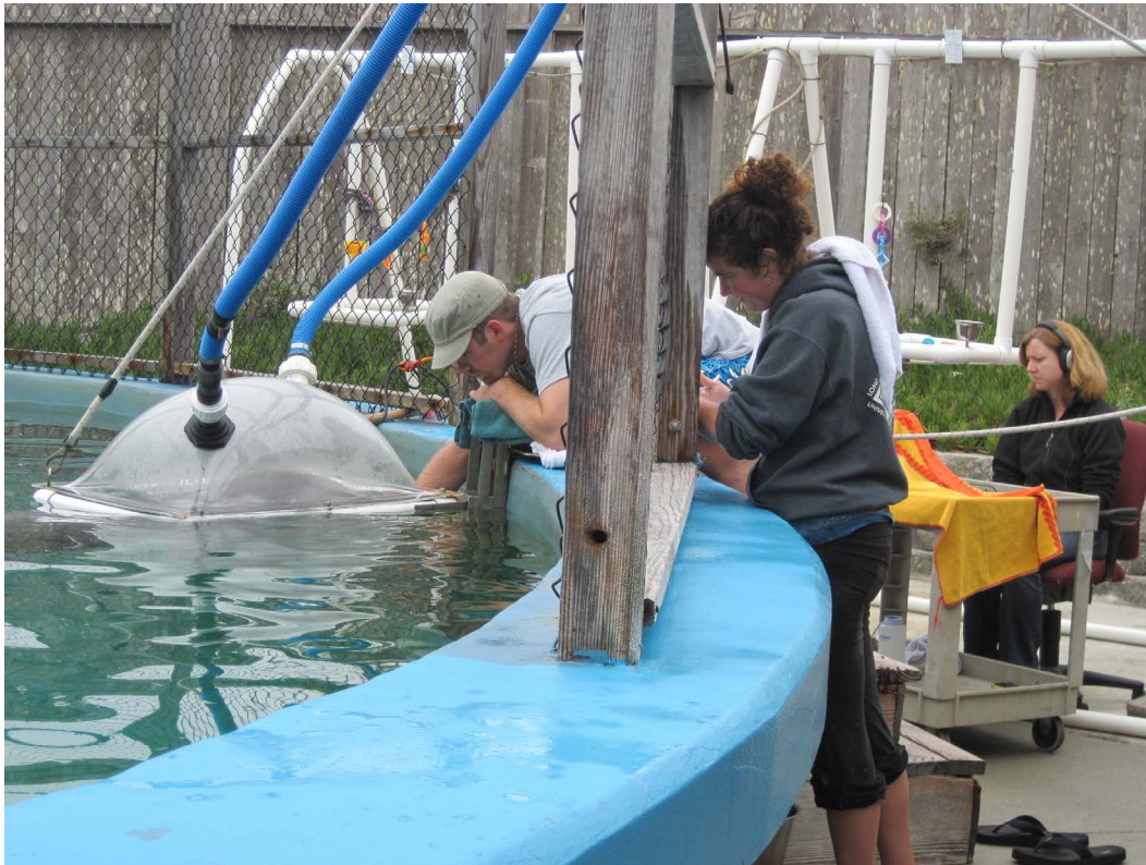
Figure 1. Photograph taken during a sound production trial showing the equipment set-up which includes the metabolic hood, the dolphin stationed under the metabolic hood, the acoustic recording equipment and operator, the dolphin trainer, and the assistant taking notes and recording respirations. During the trial dolphin clicks were recorded via a hydrophone attached to the melon by suction cup (not shown), oxygen consumption was continuously logged by an O 2 analyzer attached to a computer, and all respirations were recorded during each of the three periods.
