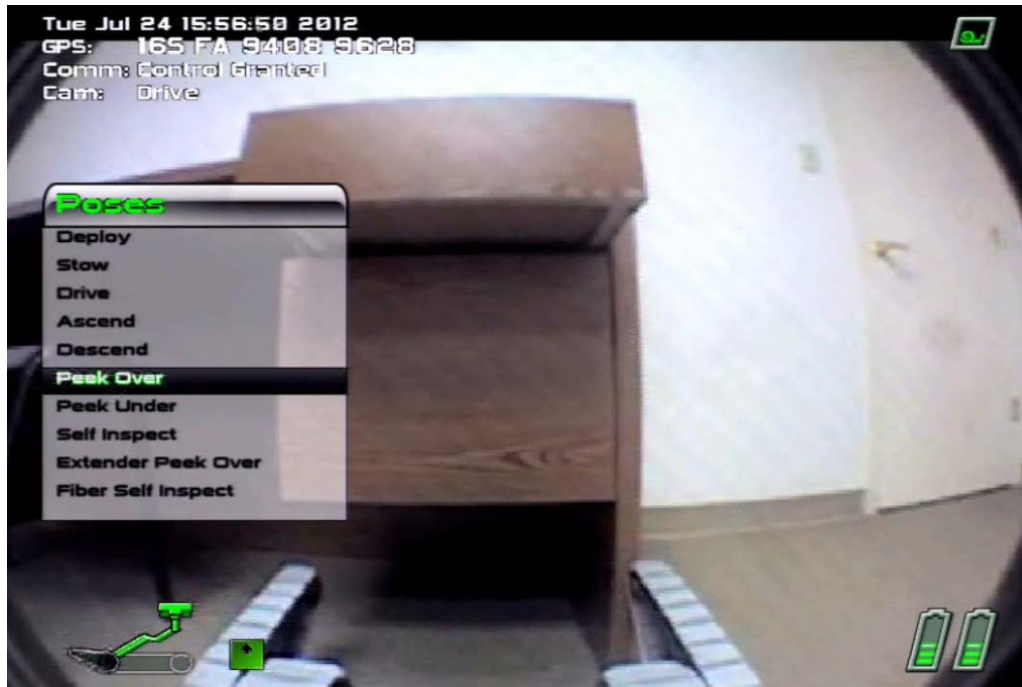
Figure 4. SUGV heads-up display showing submenu options.
