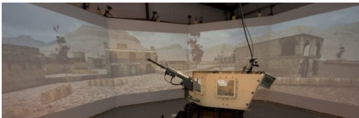
Figure 4.3 The Virtual Employment Test Bed with the GPK. Subjects target adversaries displayed on video projections upon the wrap around screens. Trigger pulls and aim on the screen are recorded. Live fire paintball guns are mounted on top of the walls. Picture by Todd Mozes.
