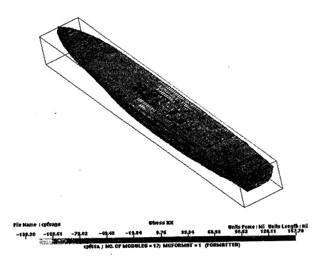
Figure 5: The MAESTRO Model Analysed with Superstructure, Showing XX Stresses in the Deck for a Sagging Load
