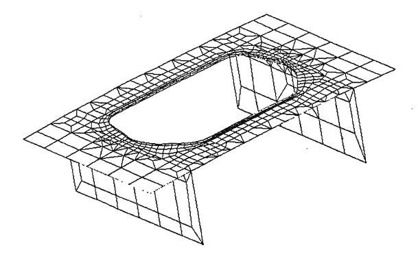
Figure 10: The Minimum Refined Model for Showing the Stresses at the Large Opening in the Deck
