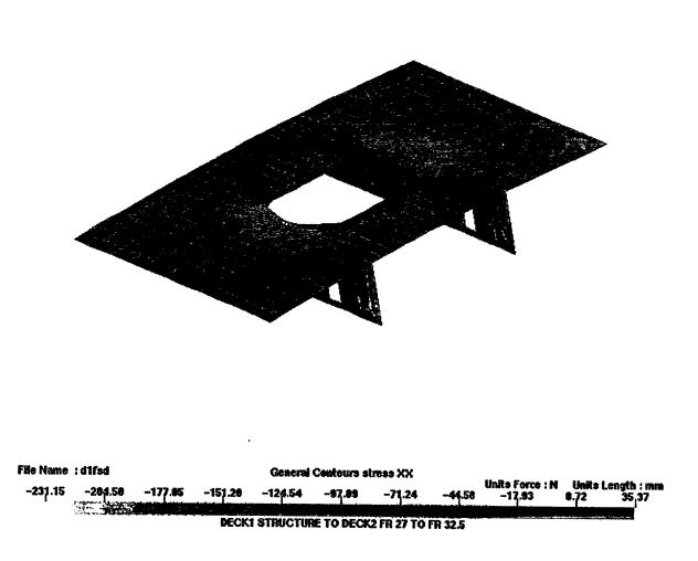
Figure 17: XX Stresses from the Top-down Analysis of the Intermediate Model of the Large Opening in the Deck with Superstructure
