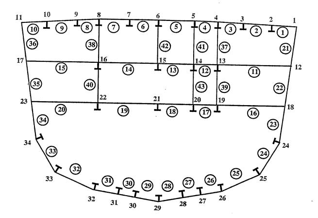
Figure 3: Midship Module Cross-section Showing the Location of the Strakes and Nodes
