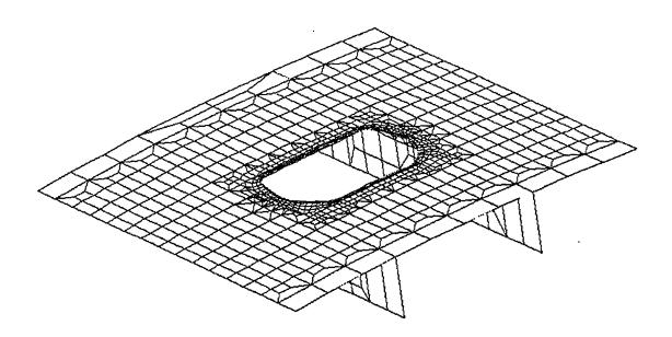
Figure 12: The Extended Deck Model with the Boundaries Nodes Adjusted to Match the MAESTRO Nodes
