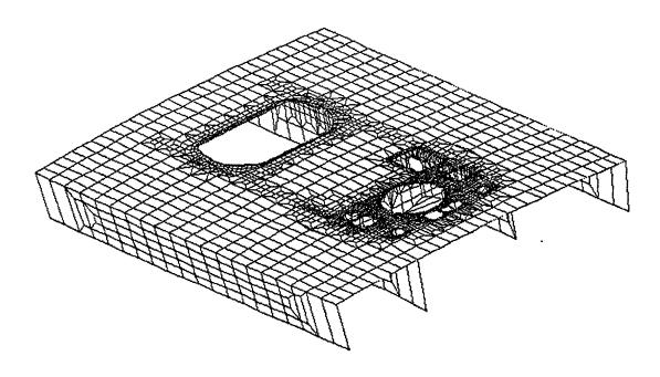
Figure 8: The Refined Grid of VAST Model of the Deck from Frames 27 to 32.5
