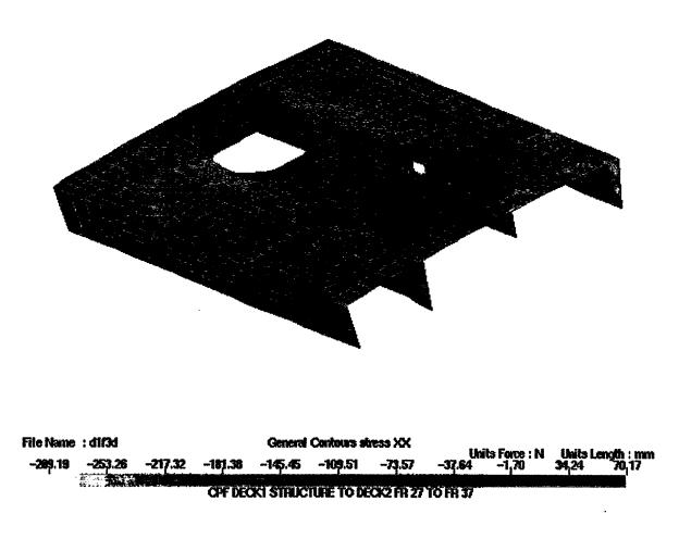
Figure 14: XX Stresses from the Top-down Analysis of the Deck Detail from Frames 27 to 32.5 with Superstructure
