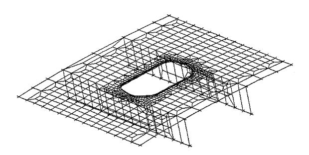
Figure 13: The Extended Deck Model Showing the Boundary Nodes
