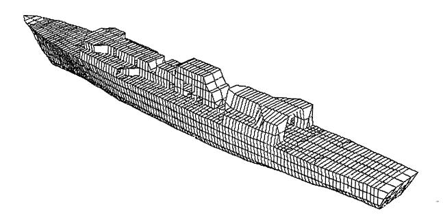
Figure 1: The MAESTRO Model of the Ship
