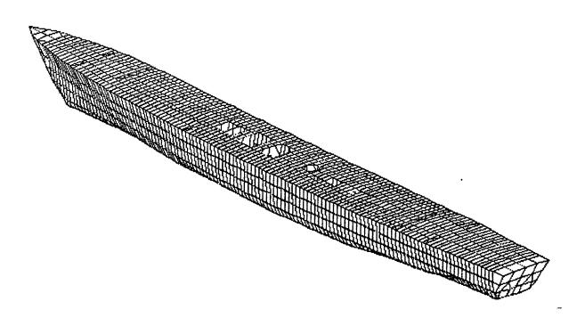
Figure 4: MAESTRO Model with the Superstructure Removed
