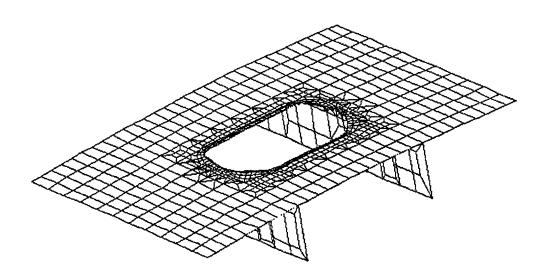
Figure 11: The Intermediate Refined Deck Model for Showing the Stresses at the Large Hole in the Deck
