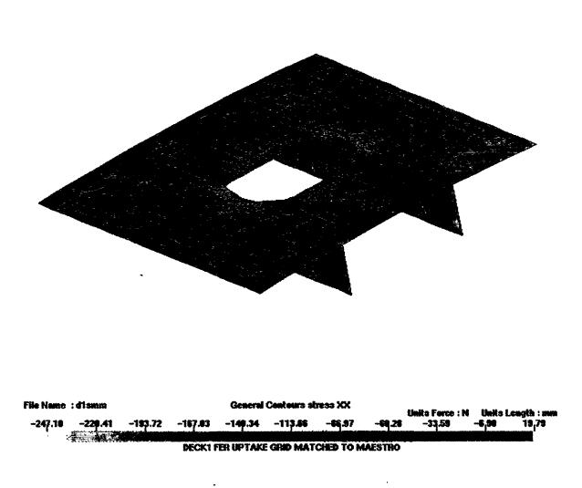
Figure 18: XX Stresses from the Top-down Analysis of the Extended Model of the Large Opening in the Deck with Superstructure
