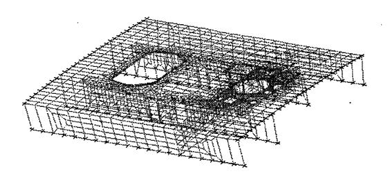
Figure 9: The Refined Grid Model Showing Constrained Boundary Nodes
