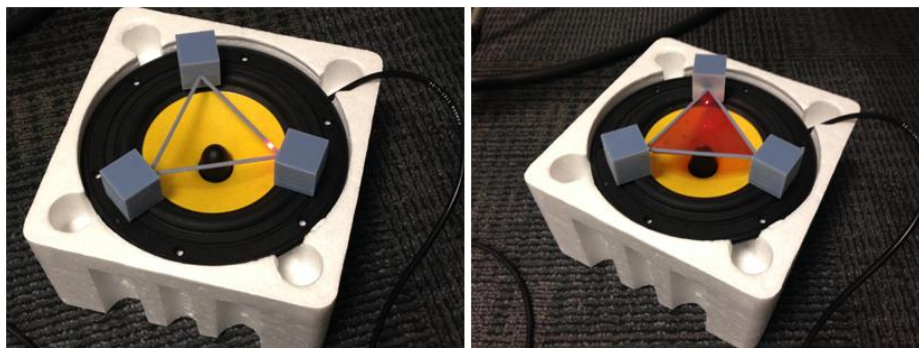
Figure 17: Test Specimen – Frame Only (Left) and Frame-Skin (Right)
