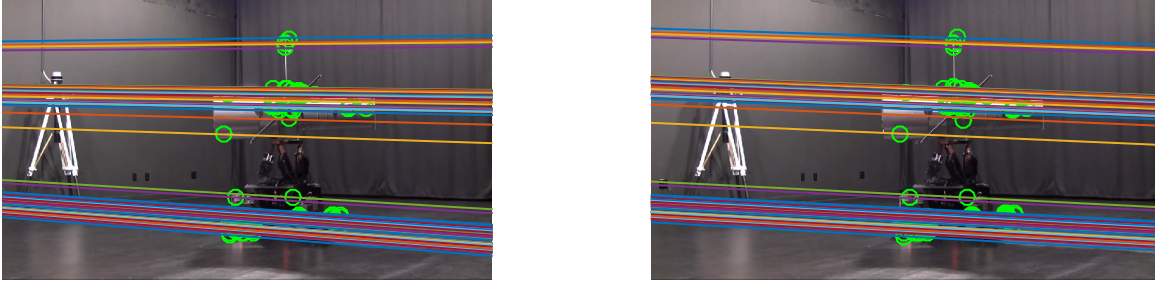
Figure 23. Epipolar Lines Shown For Fundamental Matrix Estimation.
