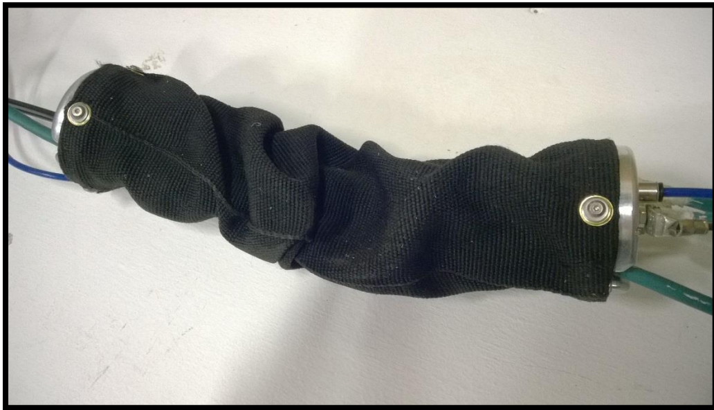
Figure 54 - Flexible pneumatic cylinder with sleeve
