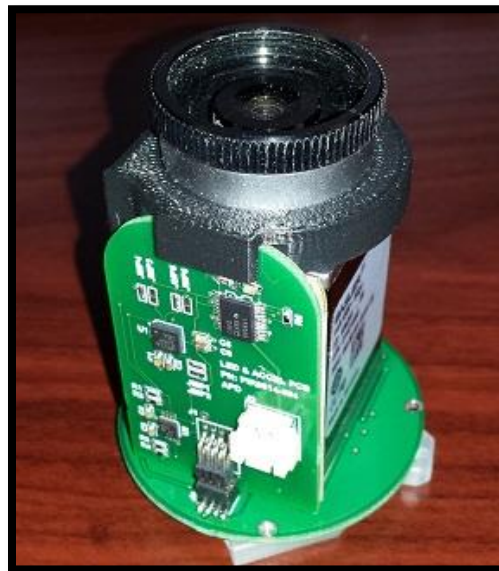
Figure 14 - Camera and associated PCBs
