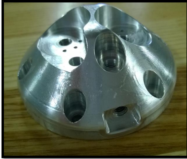
Figure 67 - Gripper cap machined under cuts
