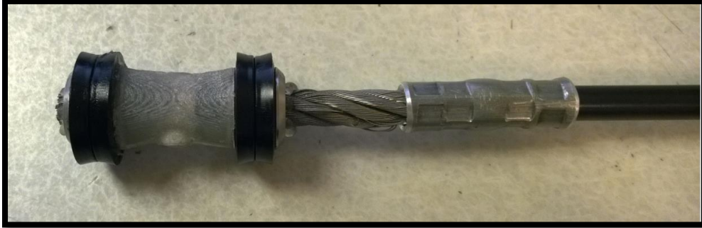
Figure 59 - Floating piston assembly with seals assembled
