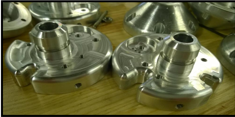
Figure 51 - Front tube cone
