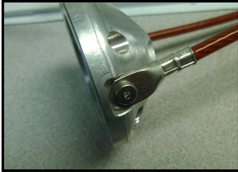
Figure 69 - Linkage fastened to gripper cap
