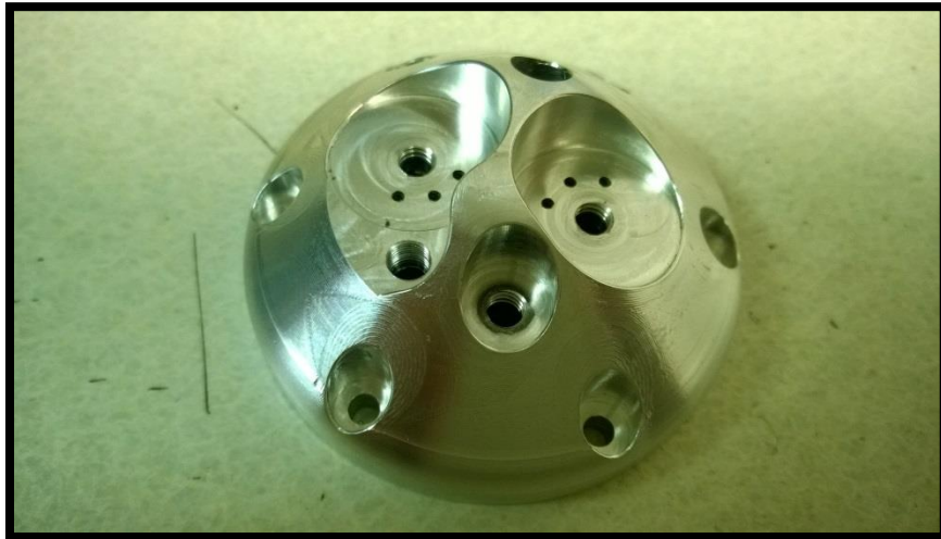
Figure 27 - Rear cone top view
