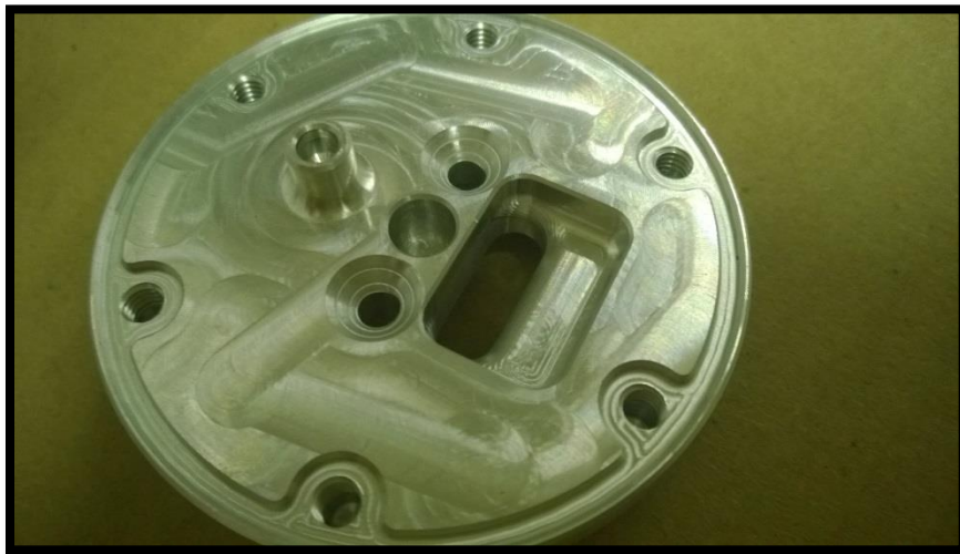
Figure 33 - Inflatable seal cap top view
