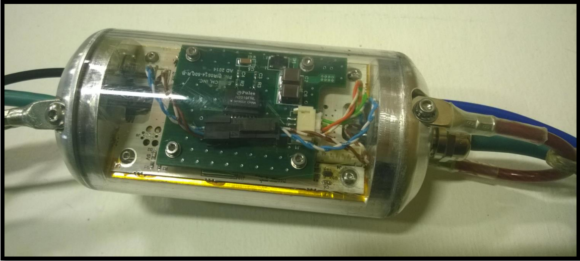
Figure 72 - Acrylic shield installed
