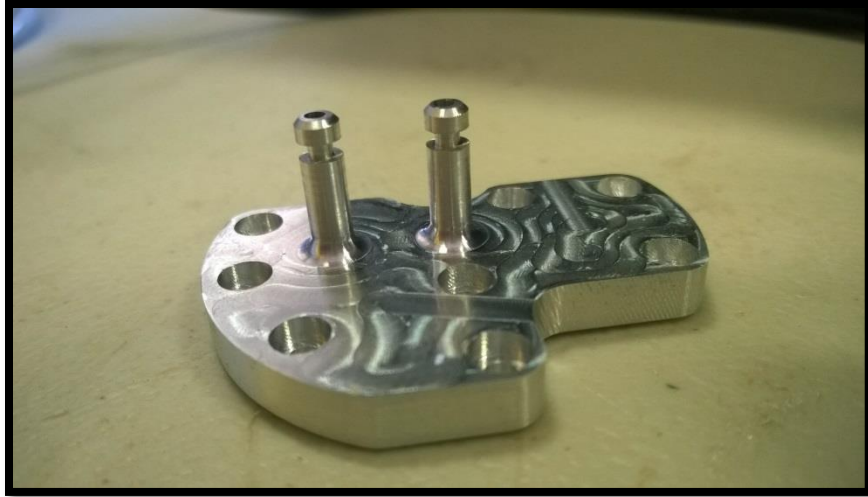
Figure 30 - Air manifold cap bottom view
