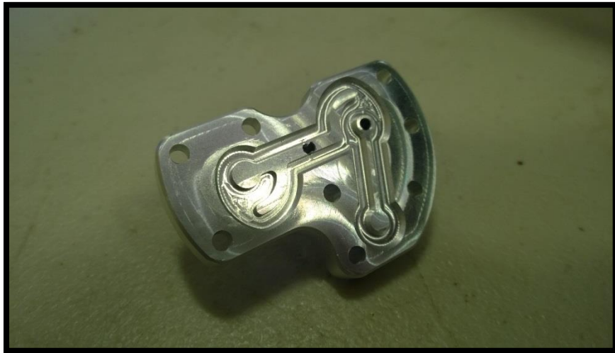
Figure 29 – Air manifold cap top view
