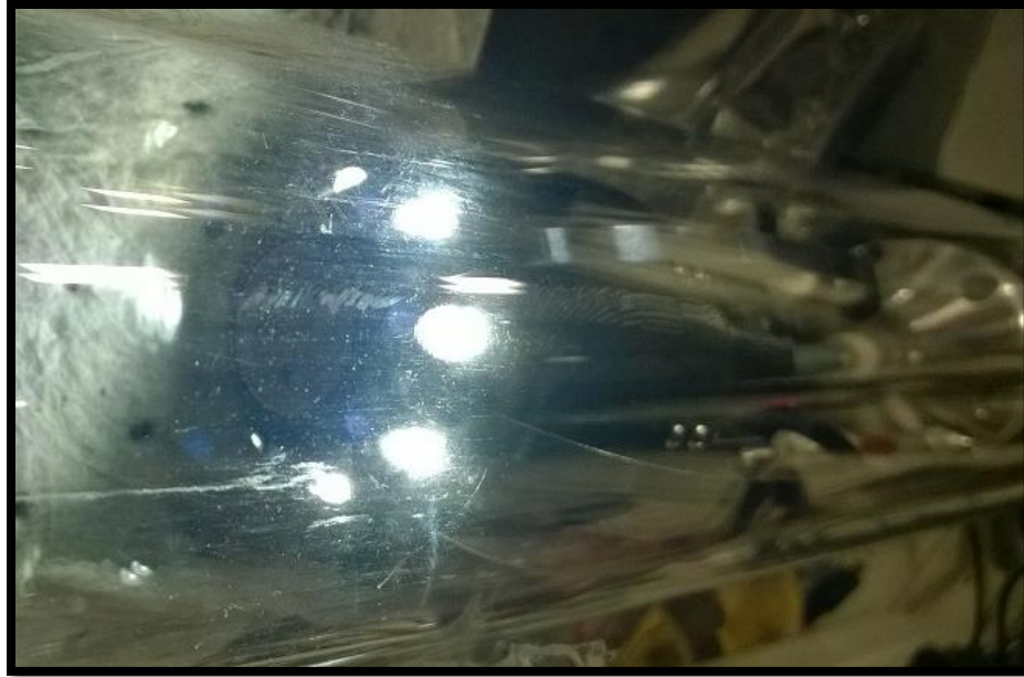
Figure 18 - Camera housing in pipe with LED's illuminated
