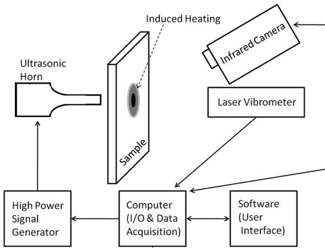
FIG. 1. Schematic of the NCATS experimental setup.
