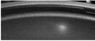
FIG. 14. NCATS imaging of a crack in aluminum wheel component.
