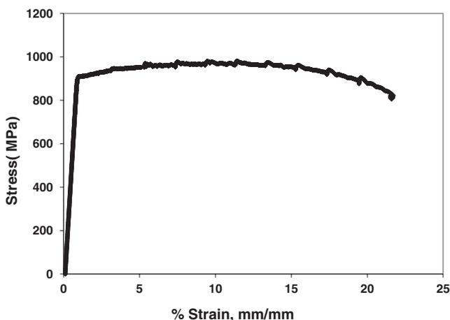
FIG. 8. Composite strain-strain curve for Ti-6Al-4V sample.
