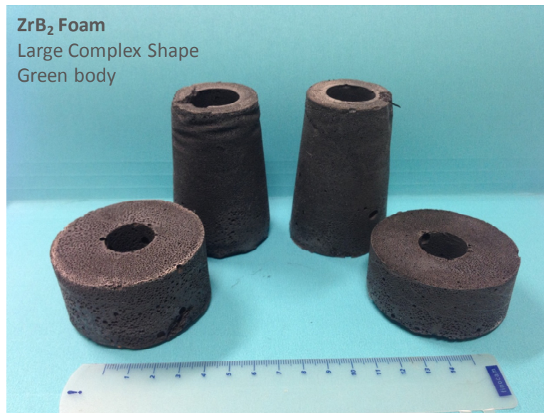
Figure 12. ZrB 2 foams produced by particle stabilized foams and gelcasting. The tapered conical cylinder was chosen to resemble the shape of a combustor.
