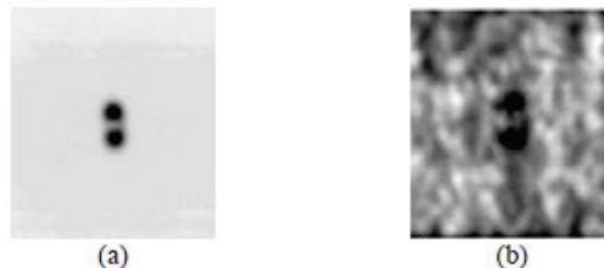
FIGURE 1. Eddy current scans taken over the same sized crack in (a) AL 2024 and in (b) Ti-6Al-4V ( \beta annealed) [1].
