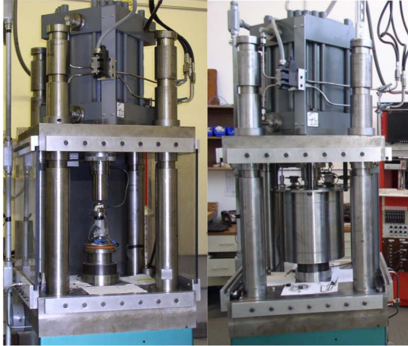
Figure 1. Hydraulic press under (left) unconfined and (right) confined operation.
